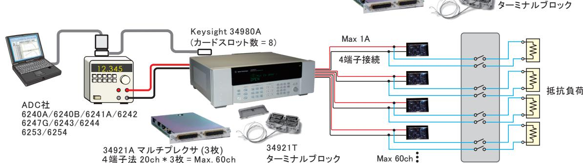
Software corresponding to a Multi-channel scanner
